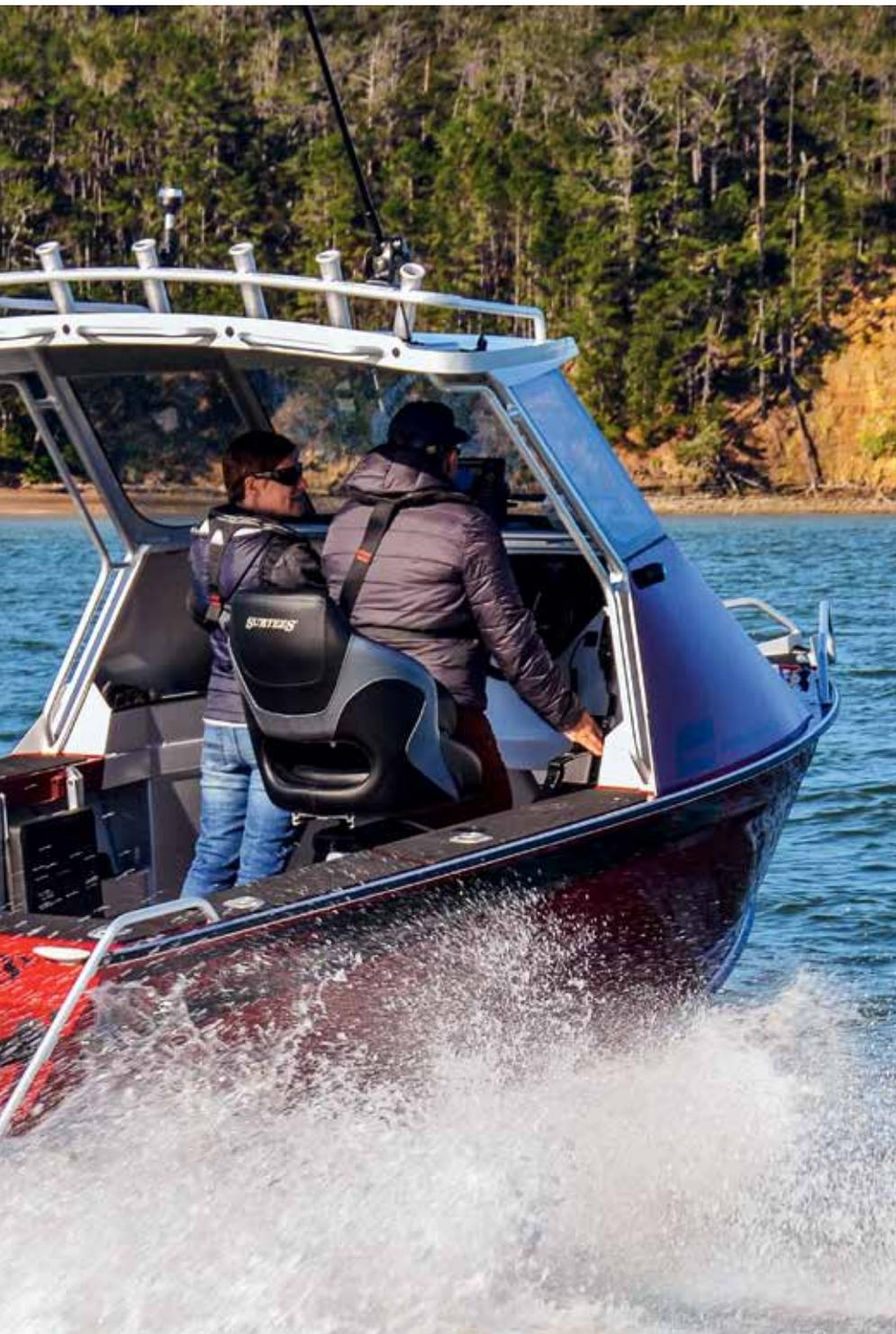
time. Wide, flat gunwales have rounded edges and are covered in cushioned foam pads to make a comfortable seat, and the gunwale and transom abound with rod-holders.
