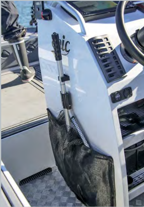
Left: Working out how to store a net in an open boat can be difficult – Surtees created this net holder, located on the side of the centre console.
