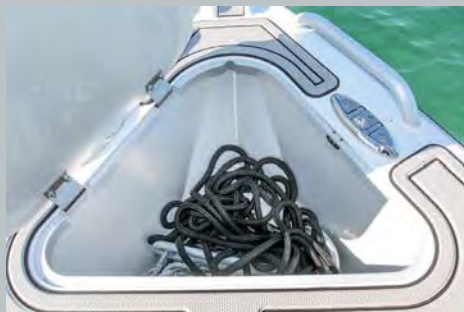
The small anchor locker, minus capstan, and diminutive fairlead were all part of the plan to keep the boat as fly-fishing friendly as possible.
