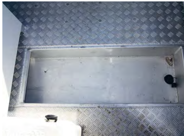
The hull framing was altered to allow for a 1.3m-long kill tank under the cockpit floor.
