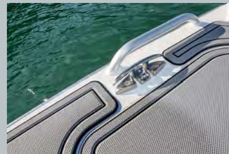
The cleats recess when not required – one less thing to catch a fly line on.
