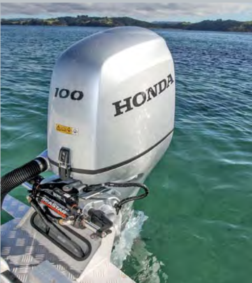
The Surtees 575 Pro Fisher is powered by a Honda BF 100hp four-stroke, making for a quiet ride with plenty of range.
