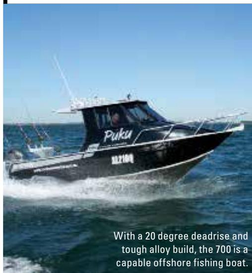
With a 20 degree deadrise and tough alloy build, the 700 is a capable offshore fishing boat.
